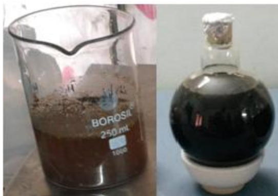
Figure 1: color change of the silver nitrate solution by the addition of the aqueous extract of A. paniculata
