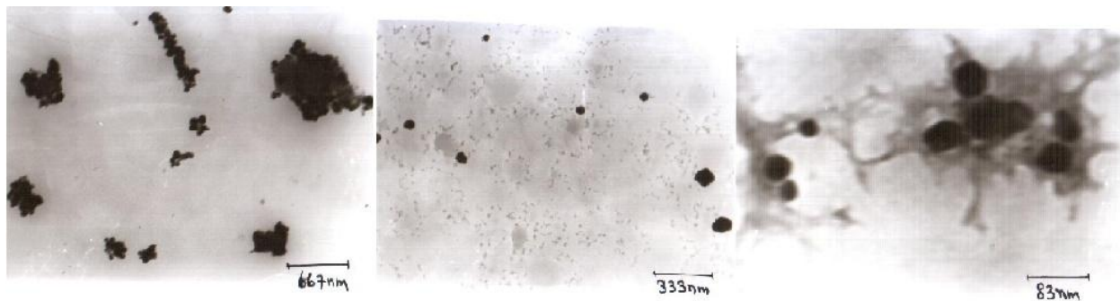
Figures 5: TEM images for the synthesized nano-particles of A. paniculata
