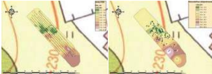
Fig. 12. Interpolated EC map with sampling points of Veris-3100 – left – and Interpolated volumetric moisture content map with TDR-300 sampling points –right –
