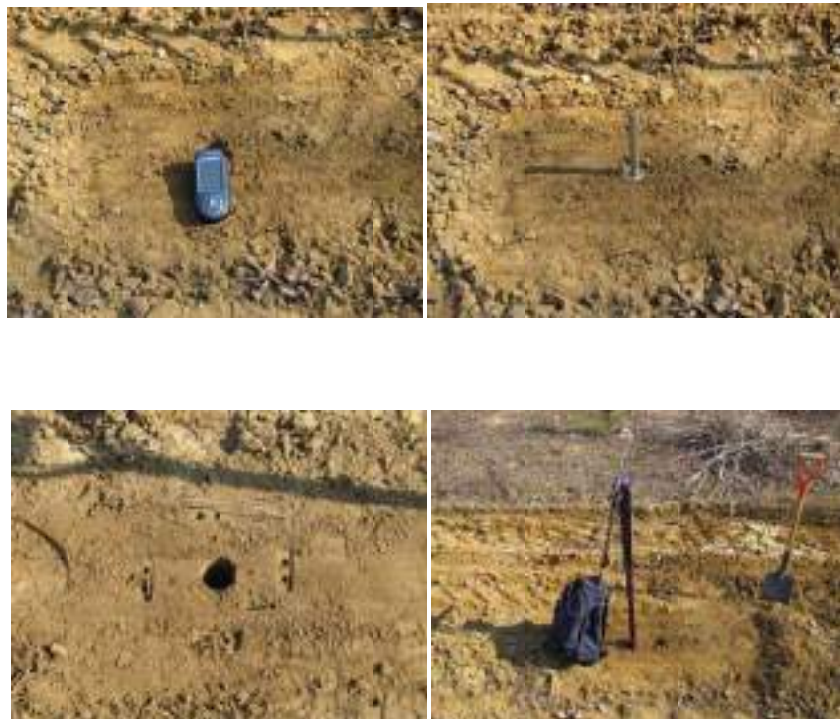
Fig. 11. Collection of soil sample, logging coordinates, measuring with volumetric moisture content with TDR-300
