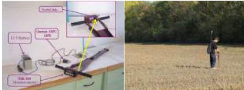
Fig. 10. The Spectrum TDR-300 soil moisture meter and its utilization
