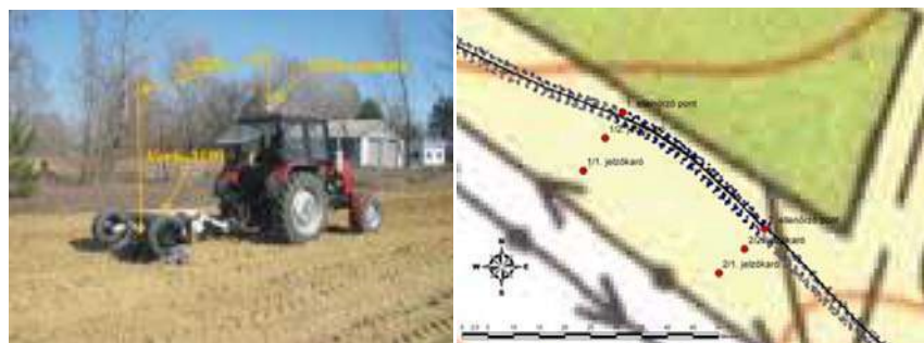
Fig. 9. Distance between the GPS antenna and measuring disks of Veris-3100 and the validation method
