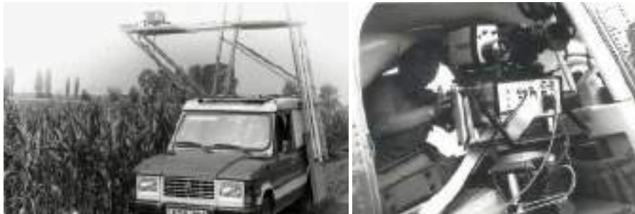
Fig. 3. Thermal evaluation of maize and thermovision assembly on a chopper
