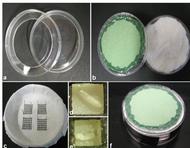
**Figure 2.** Fecundity box. (A) Plastic Petri dish and lid with a concentric opening. (B) Plastic Petri dish filled by pressed cotton and lid with a concentric opening covered by a piece of glued cotton tissue. (C) Top of the fecundity box showing the filter paper covering the cotton layer and the four mosquito net fragments. (D) Detail of a mosquito net square showing an unhatched egg. (E) Detail of a mosquito net square showing a hatched egg. (F) Overview of the assembled fecundity box.
