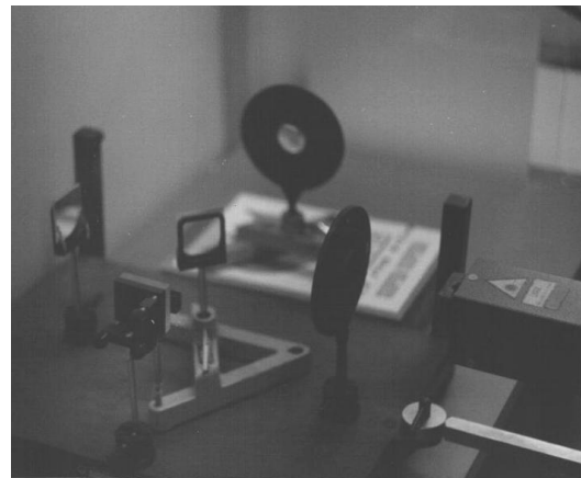
Figure 1. It is schematic diagram of the Twyman-Green interferometer set up and a photo of the lab for measuring progressive addition lenses.
